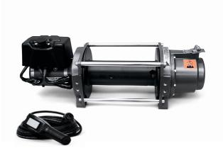
The Series 9 DC features a weatherproof industrial contactor and heavy duty remote control. The disc brake is designed for extended power-out use and the motor is protected by a thermal over-load switch. Its lower gear ratio of 199:1 provides a fast line speed. Designed to meet SAE J706 and CE standards.
