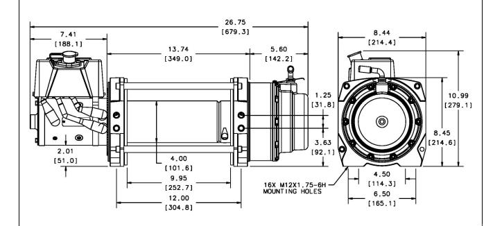
Motor / Contactor may be rotated in 90 degree increments. Clutch housing may be rotated in 72 degree increments.
