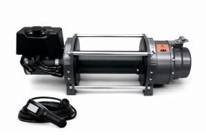
The Series 15 DC features an extended run time high powered DC motor with a weatherproof industrial contactor and heavy duty remote control. The disc brake is designed for extended power-out use. Designed to meet SAE J706 and CE standards. The motor is protected by a thermal overload switch.
