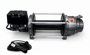
The Series 12 DC features a weatherproof industrial contactor and heavy duty remote control. The disc brake is designed for extended power-out use and the motor is protected by a thermal over-load switch. Designed to meet SAE J706 and CE standards.
